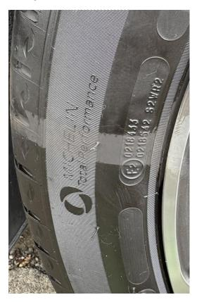
Turtle Wax® on top, control in the middle, Acrylic Tire Shine on the bottom. Substrate was MICHELIN Total Performance tire on 2025 Lincoln Corsair.
